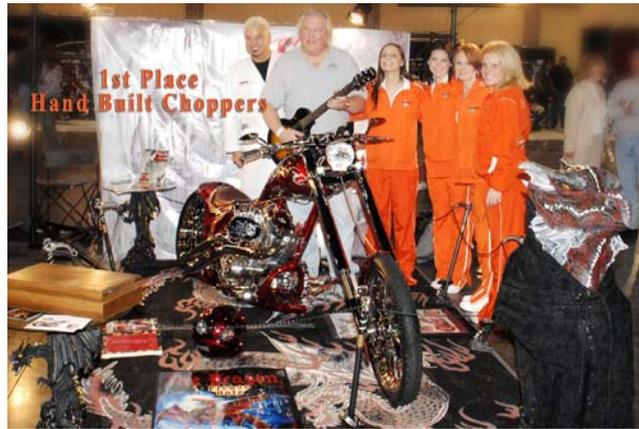
Johnson 133 cu. in. engine with two Minkuni carbs. Power flows through a Baker six speed to an Eddie Trotta single side swing arm before reaching the massive 280 rear tire
